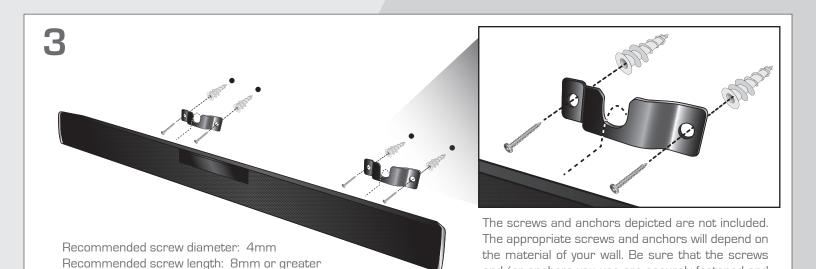
Attach the brackets to the wall as shown. Gently hang the Sound Bar on the brackets using the wall mount posts on the back of the Bar.
